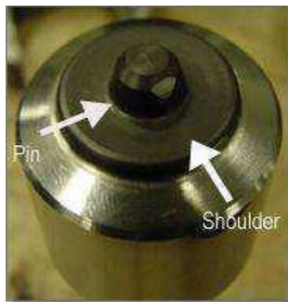
Figure 1.8 Pin and Shoulder of FSW
