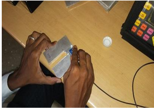
Figure 3.13 Non destructive testing for FSW welded region
