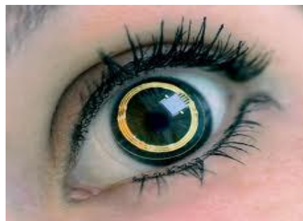
Fig.1.5. Implantable pressure sensor to measure Intraocular Pressure (IOP)
