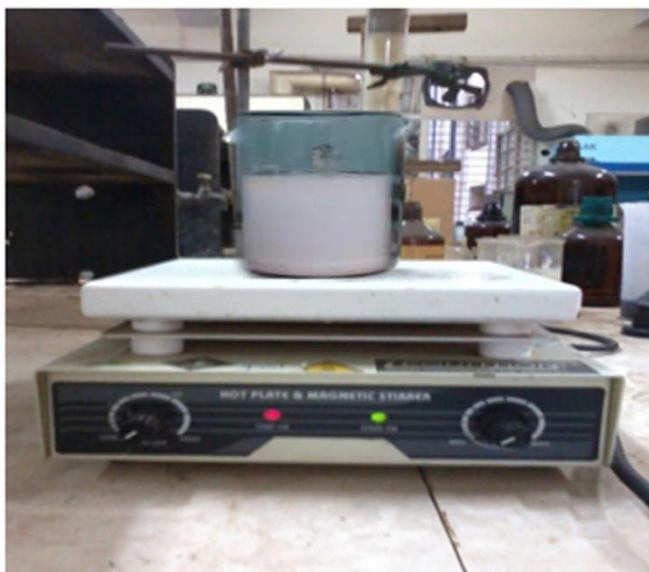
Figure 3.4 Preparation of titanium di-oxide nanofluid using magnetic stirrer cum hot plate
