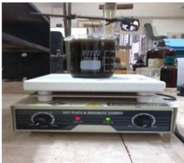
Figure 3.10 Preparation of copper oxide nanofluid using magnetic stirrer cum hot plate
