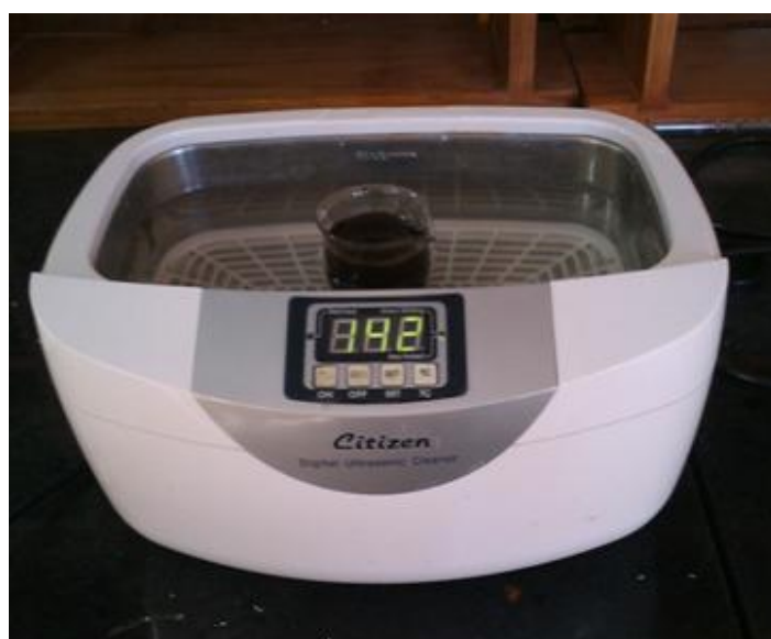
Figure 3.11 Ultrasonication of copper oxide nanofluid
