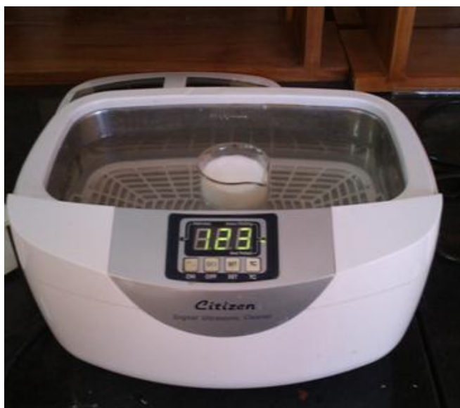
Figure 3.5 Ultrasonication of titanium di-oxide nanofluid
